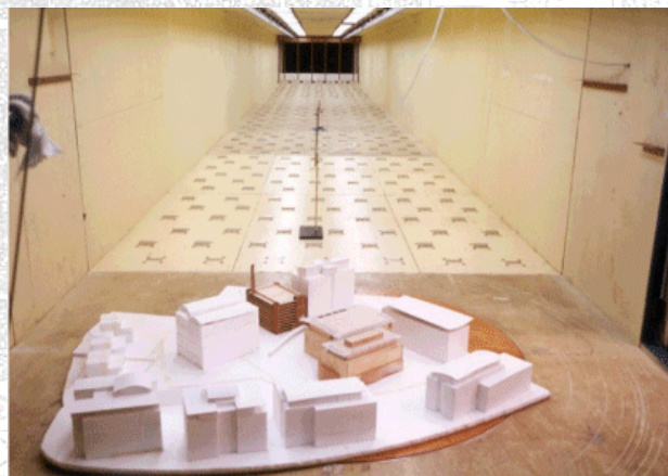
Figure 7: Wind Velocity Tunnel Testing
